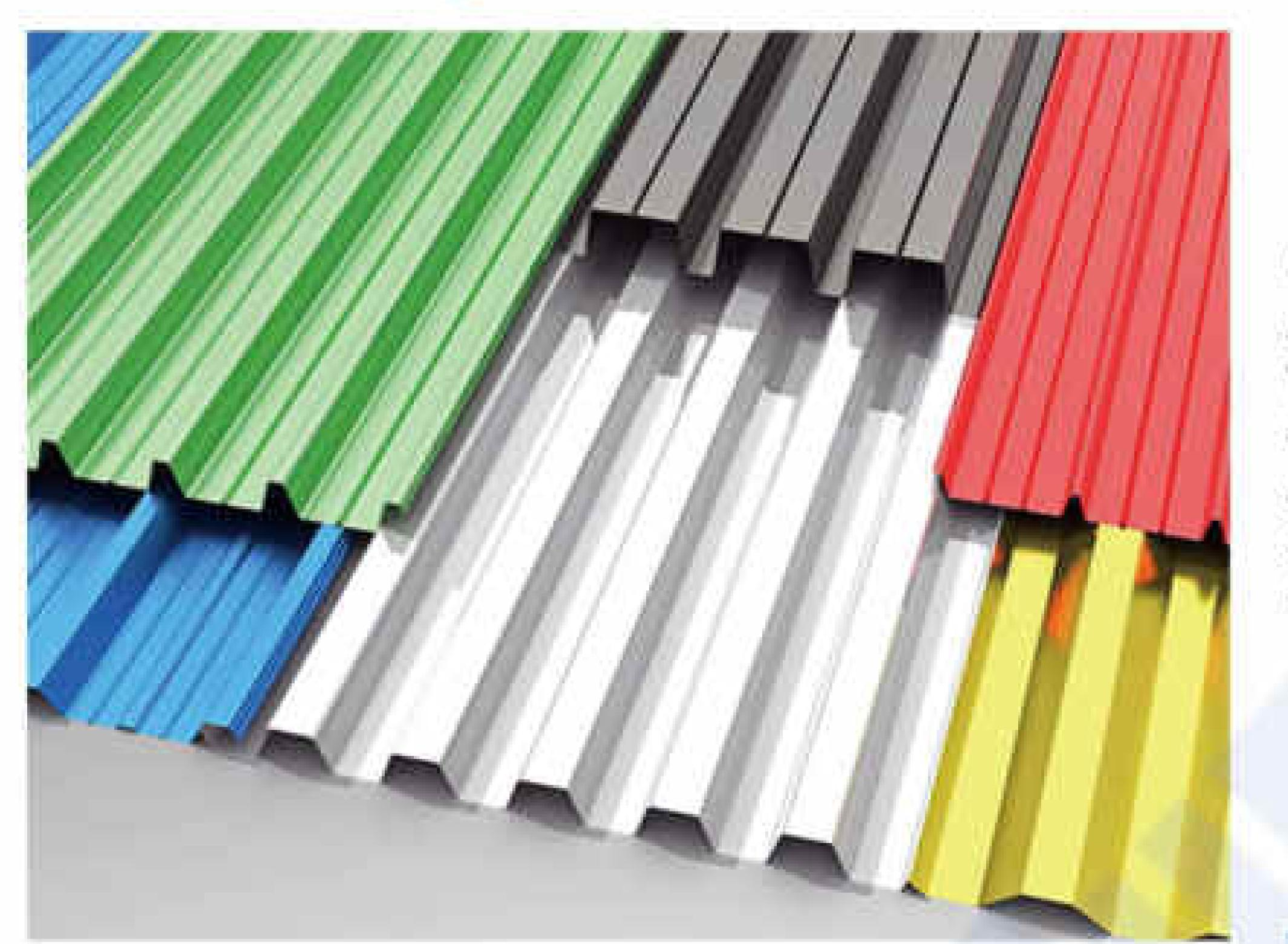
Corrugated metal roof is using color coated steel or aluminum alloy metal sheets and cold-rolled into various profiled sheets by rolling equipment. Corrugated metal roof or steel sheets are an energy-efficient, low cost, and long-lasting roofing and wall cladding option for homes, log cabins, and commercial building envelope applications.
